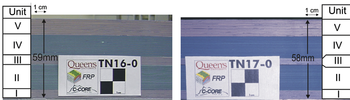
Fig. 4. Initial configurations of models TN16 and TN17, each composed of five internally layered stratigraphic units of alternating bulk competency, with an incompetent unit at the base (labeled as units I through V). Table 2 details the layer compositions and thicknesses.
